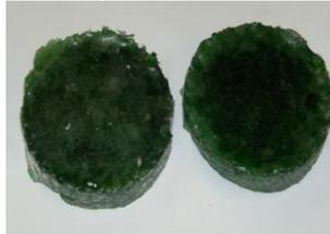
Fig.2 Opaque glass brick without metal shell
