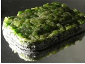
Fig. 6. Rectangular non-smooth glass brick produced by fusing in a sardines' can mould (Photo taken by Mr H. Hills, SET, UoB)
