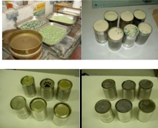
Fig.6. Stages of RG's 1<sup>st</sup> sieved granulated glass, 2<sup>nd</sup> after placed the tin can, 3<sup>rd</sup> after placed the lid, 4<sup>th</sup> after placed the appropriate weight on the top of the lid before put in the oven.
