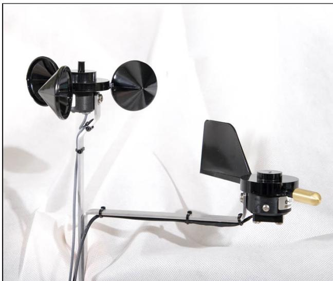
**Figure 9.3** Anemometer and wind direction vane
