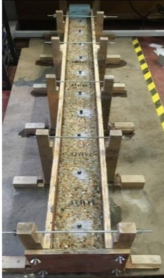
**Figure 3** Beam with dowels ready for casting
