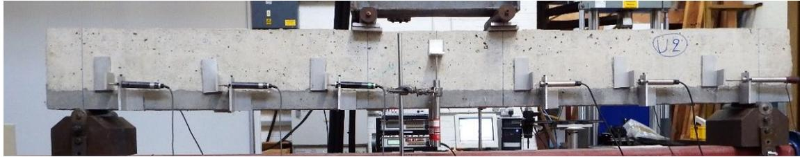
**Figure 5** Experimental setup for the testing of beams
