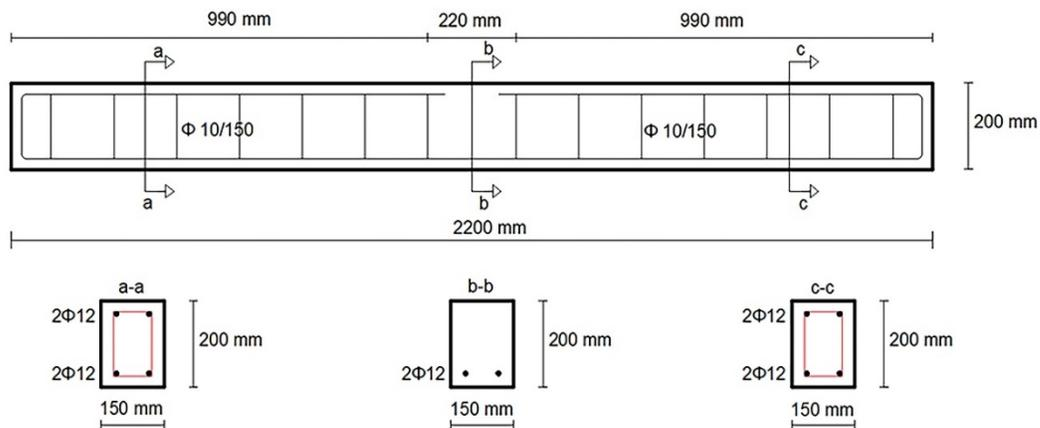
**Figure 1** Geometry and reinforcement of the RC beams
