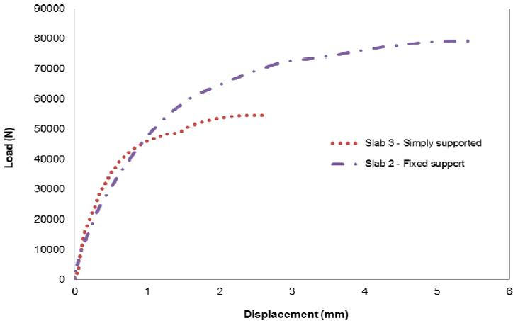
**Fig. 3** Load-deflection curve for one of the slab specimens.
