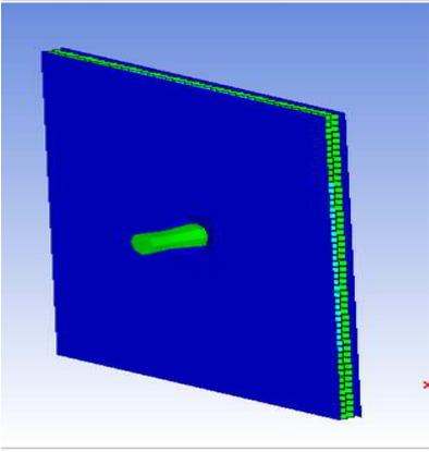
**Fig. 5** Impact on the slab that has steel plates as additional reinforcement.
