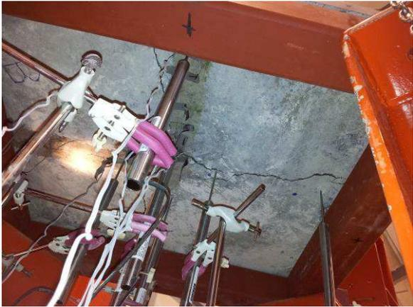
**Fig. 2** LVDTs arrangement for the static test.
