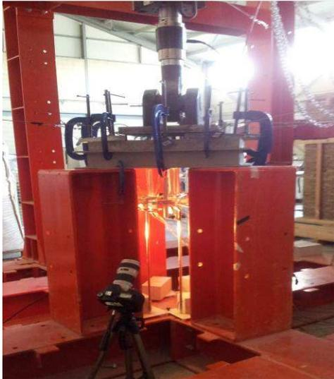
**Fig. 1** Experimental set-up for the static tests in UHPFRCC slabs.
