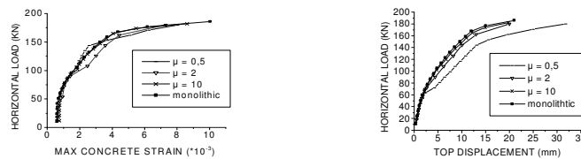
Figure 2: Maximum concrete strain and top displacement against horizontal load for differing values of \mu and a constant c equal to 1MPa.
