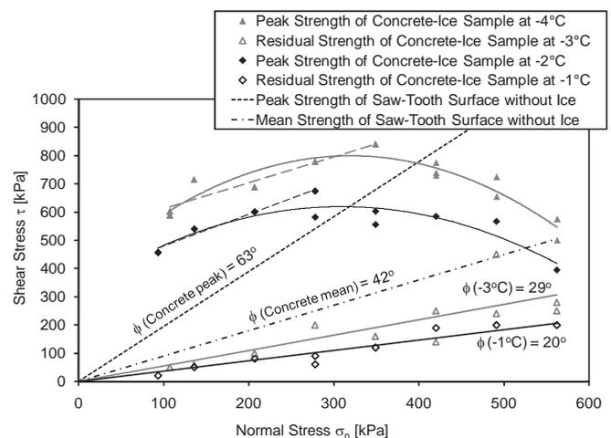
Figure 1. Peak shear strength and residual shear strength results of concrete-ice samples and saw-tooth surfaces without ice.
