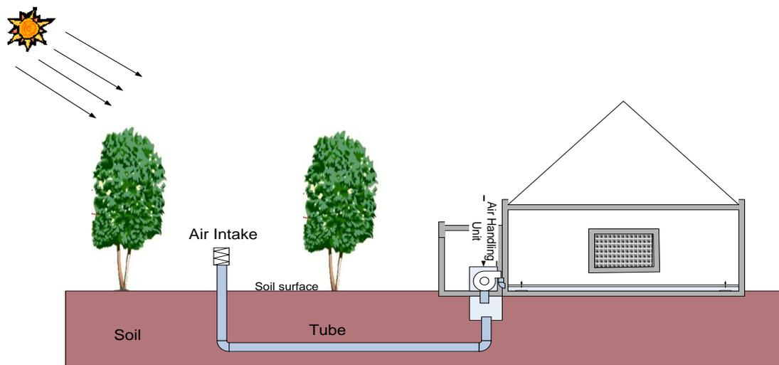
**Figure 1 Configuration of Earth-air heat exchanger**
