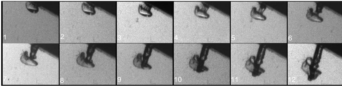
**Figure 3.** Ultra-high-speed video of a fossil diesel jet injected at 40 MPa into atmospheric conditions.
