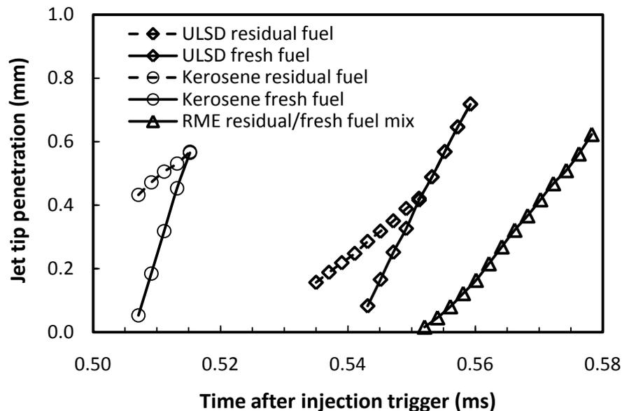
**Figure 4.** Injection timing of kerosene, fossil diesel and RME fuels injected at 40 MPa into atmospheric conditions. The plots for the fossil diesel were obtained from the video presented in Figure 3.
