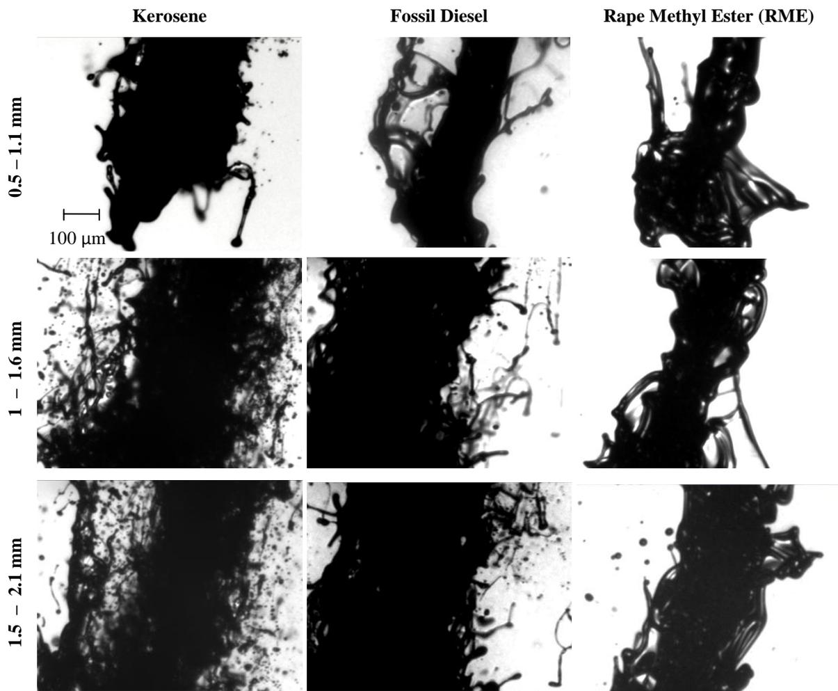
**Figure 5.** Morphology of the jet at/near the leading edge of the spray up to 2.1 mm below the nozzle. Each row represents the same spatial location. 40 MPa injection pressure sprayed into atmospheric conditions.
