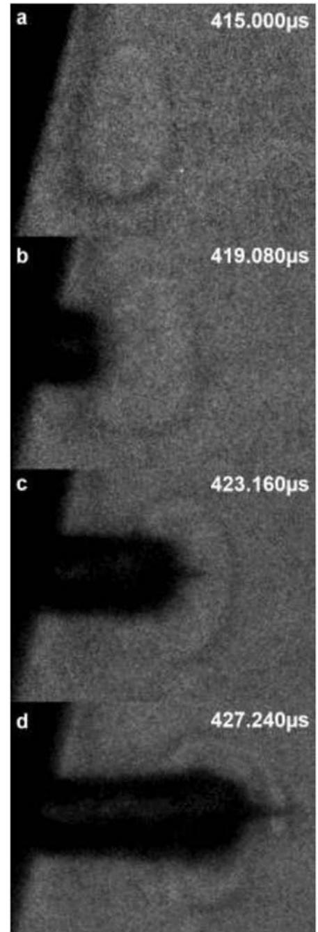
**Figure 3. Perforation of the vapourised spheroidal cap by a liquid jet, indicating the presence of a vortex ring structure inside the cap. A central ligament is formed and propelled ahead of the main jet.  $P_{inj} = 40$  MPa; ICP = 4 MPa. Timings are relative to start of injection trigger pulse.**
