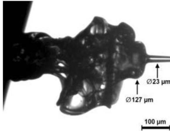
Figure 4. 23  $\mu\text{m}$  central ligament propelled ahead of the jet by the vortex ring motion in the spheroidal cap. The jet seen in Fig. 3d at the base of the ligament is also visible here with a diameter of 127  $\mu\text{m}$ .  $P_{inj} = 40 \text{ MPa}$ ;  $ICP = 0.1 \text{ MPa}$ .
