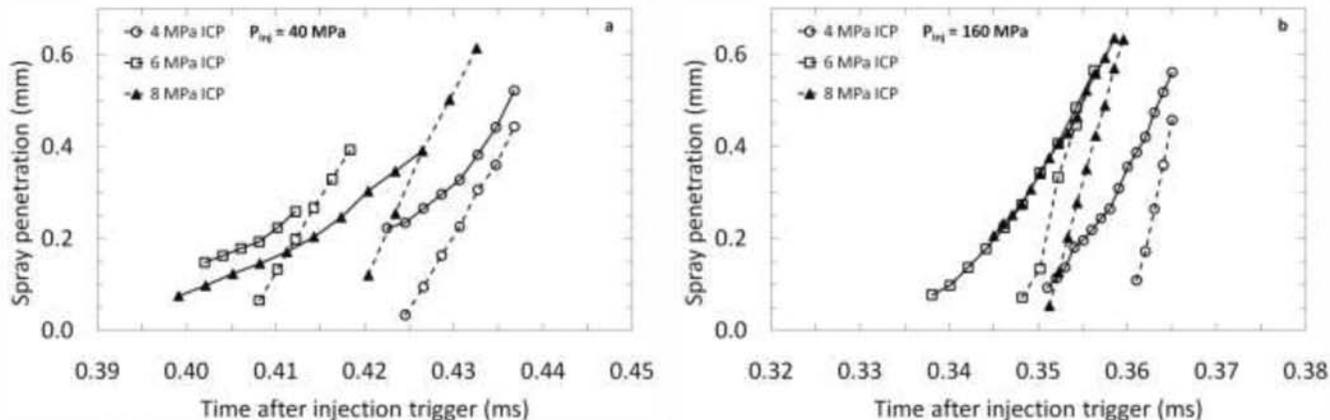
**Figure 7.** Initial spray penetration for 40 (a) and 160 MPa (b) injection pressure and a range of ICPs. Solid lines represent the vapourised spheroidal cap's penetration, and the dotted lines the liquid jet's.
