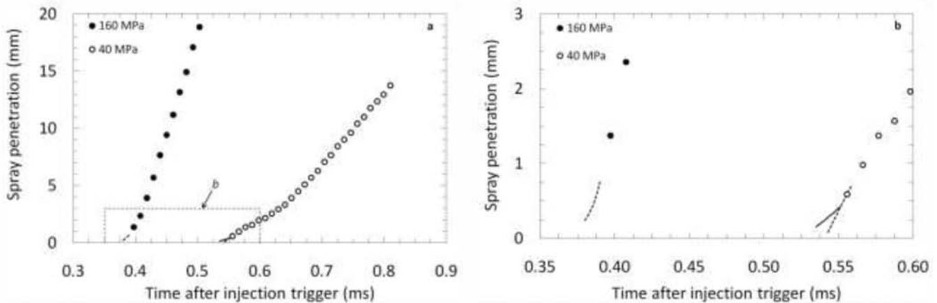
Figure 5. Evolution of liquid spray penetration with time for 0.1 MPa ICP (atmospheric condition) and two injection pressures, recorded at macroscopic (a) and microscopic (b) scales simultaneously. Solid lines represent the spheroidal cap's penetration, and the dotted lines the liquid jet's.
