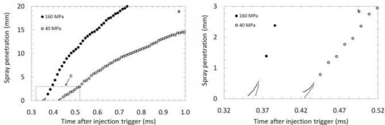
**Figure 6.** Evolution of liquid spray penetration with time for 4 MPa ICP, recorded at macroscopic (a) and microscopic (b) scales simultaneously. Solid lines represent the spheroidal cap's penetration, and the dotted lines the liquid jet's.
