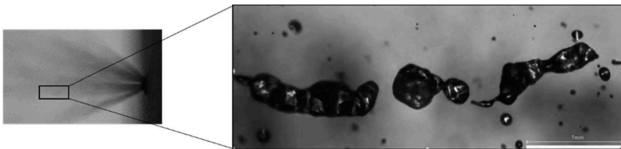
Figure 4. LN 2 spray into ambient air. The left image shows the spray in whole. The right image is the magnified image of the location marked by black rectangle in the whole spray.
