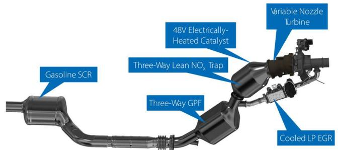
Figure 7 Layout of the aftertreatment system
