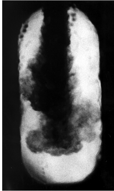
Figure 6. Injection at 160 MPa; photograph taken 4.95°CA after start of injection; pressure at TDC: 8 MPa; spray penetration about 4.5 cm.
