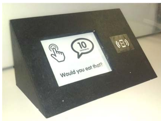
Figure 1: Deployed displays consisting of a 6 inch e-ink screen and black casing to fit in with gallery environment.
