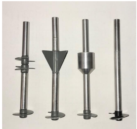
Figure 2. Model screw piles with enhancements.
