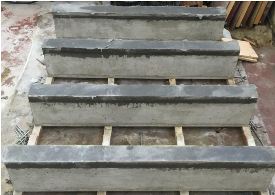
Figure 6. RC beams a) before and b) after casting of the strengthening layer.
