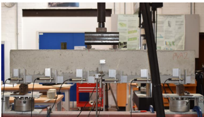
Figure 12. Experimental set up showing the distribution of LVDTs for RC beams.
