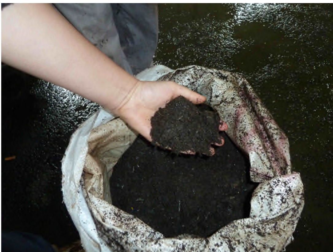
Figure 10: The finished product after 8 hours in the biological digester
