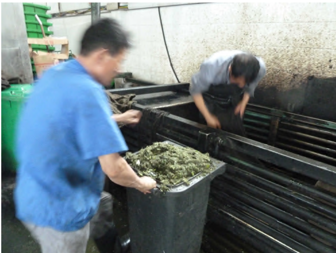
Figure 9: Ground food waste being placed into the compressor for water extraction
