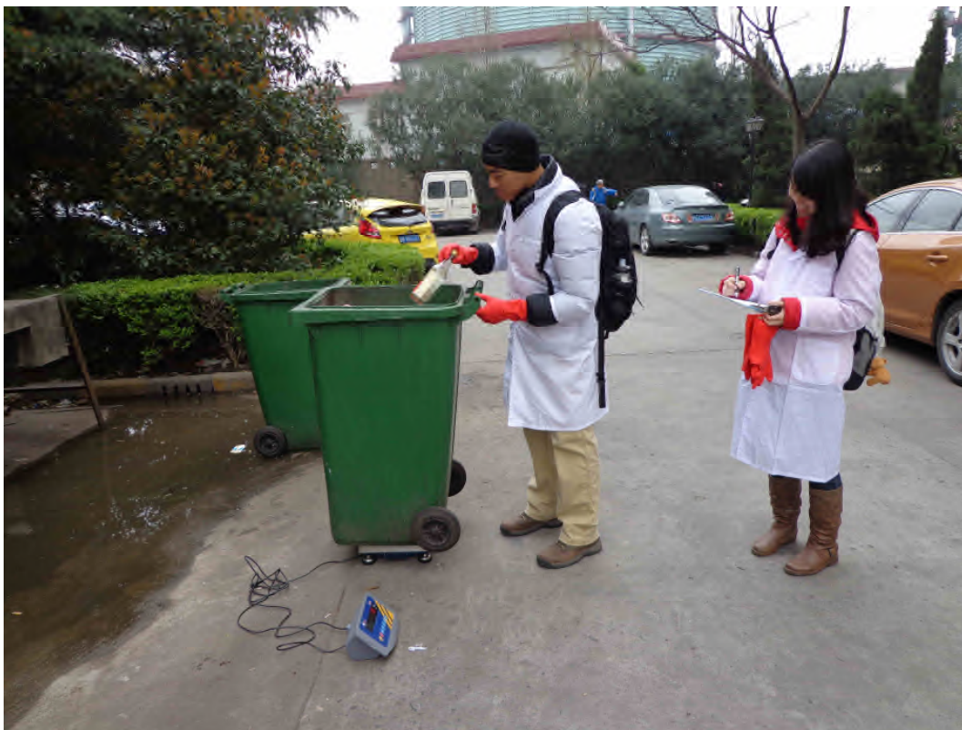
Figure 17: Bin weighing processed used in Ying Hua Yuan
