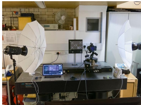
Figure 4-4. Image of camera positioning robot with camera, DICE target, and Bowens studio strobes in place.
