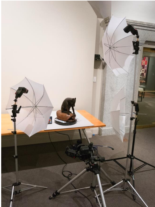
Figure 6-19. Imaging setup with positions of three Canon Speedlite flashes and object on turntable.
