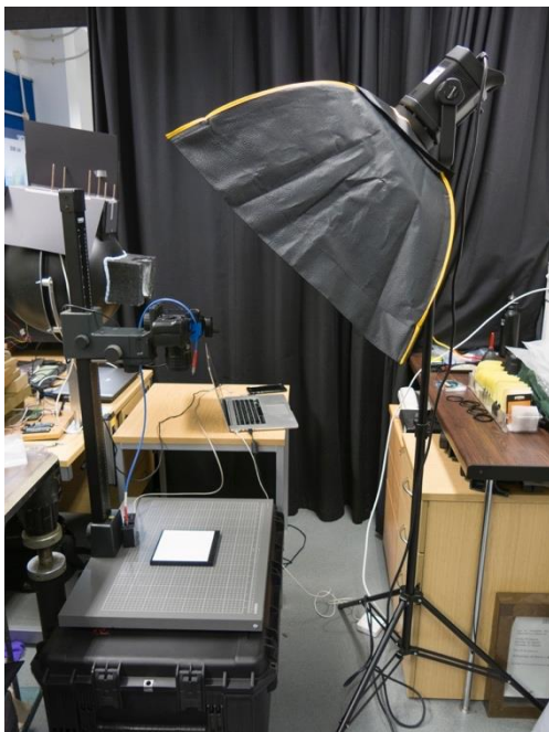
Figure 14-10. Setup for spectral response measurement (Iteration#4) with a single Bowens strobe.
