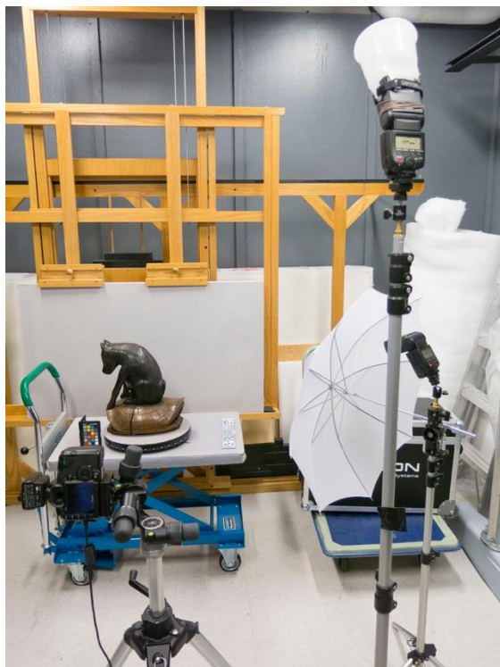
Figure 6-26. Imaging setup in the Lunder Conservation Center that shows the position of the lights to the right of the camera.
