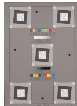
Figure 1-4. DICE device level target (17.9 x 25.4 cm) used for assessing 2D image quality and performance.
