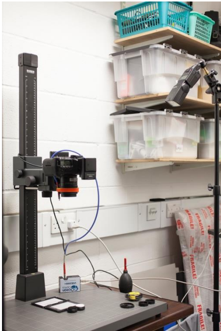
Figure 14-9. Setup for spectral response measurement (Iteration#3) with a single Canon Speedlite flash.
