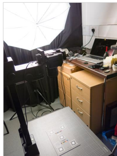
Figure 6-2. Image of setup for filtered camera acquisition.
