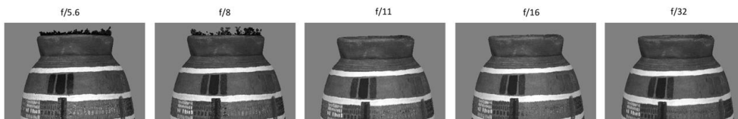
Figure 7-13. Detailed views of resulting models from the DOF-3D-MangoVase test. The datasets acquired with the smallest DOF (f/5.6 and f/8) resulted in artefacts around the rim of the vase while the datasets acquired with a larger DOF were able to better record the rim and interior of the rim of the vase.
