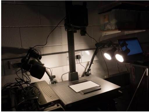
Figure 14-7. Setup for spectral response measurement (Iteration#1) with tungsten lamps and copy stand.
