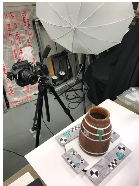
Figure 4-16. Imaging setup with Mango Vase test object on turntable. The camera is mounted on a tripod and one of the two flashes with umbrellas is seen in the image. CHI scale bars are positioned on the turntable around the object.
