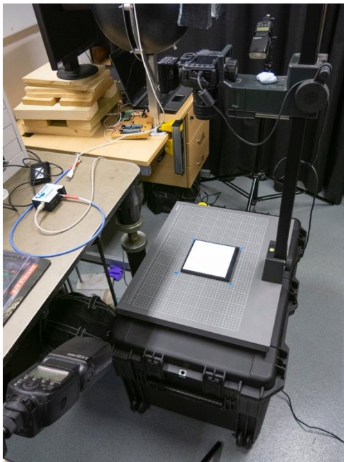
Figure 14-8. Setup for spectral response measurement (Iteration#2) with two Canon Speedlite flashes. The copy stand was positioned on a pelican case in order to have the flashes positioned on each side of the setup.
